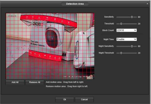
**Sensitivity**: Higher sensitivity will consider minor changes as motion. Lower sensitivity will require more significant changes to be considered motion. Set the sensitivity of the motion detection. **Threshold**: Higher threshold means that more "blocks" needs to contain motion in order to trigger an alarm. Lower threshold means that less "blocks" needs to contain motion in order to trigger an alarm.
